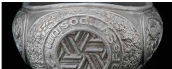
Figure 18 Cast result of a heat-cured signet ring
