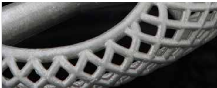
Figure 15 Cast result of a heat-cured cage ring
