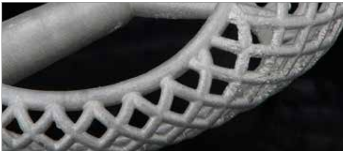
Figure 14 Casting result of a UV-cured cage ring
